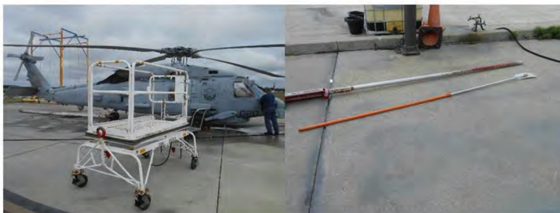
Figure 6. B-4 stand observed at the wash rack to access and wash the top of the aircraft (left) and telescoping brush poles (right).
