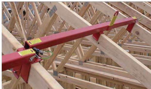
Anchorage connector for wood construction that spreads the fall forces on more than one rafter
