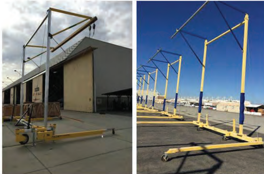
Figure 11. Examples of mobile, horizontal rail systems.
